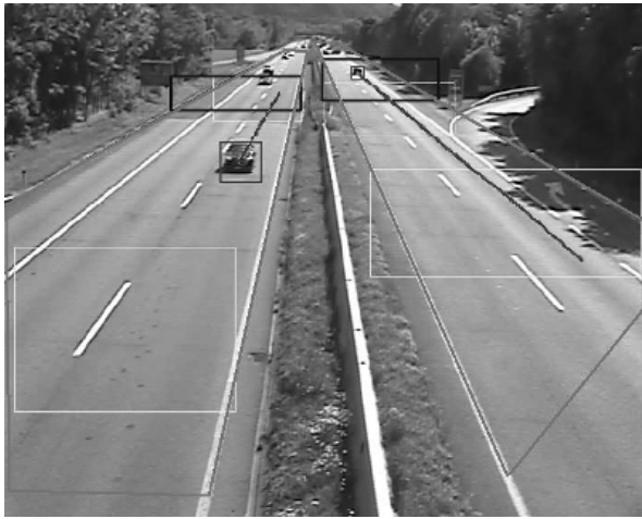
Fig. 3. Video-based vehicle tracking. Detection area indicated in white, tracking area in light grey, long-distance tracking area in black and the actual vehicle tracks are in dark grey.
