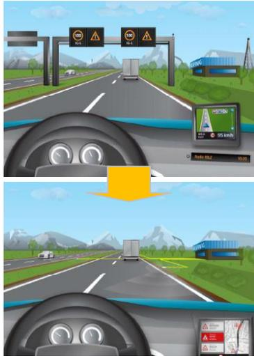
**Figure 1.** Top: current situation (information is distributed to road and in-car HMI). Bottom: ASFINAG vision of future V2I safety systems (all information is provided by the in-car HMI).
